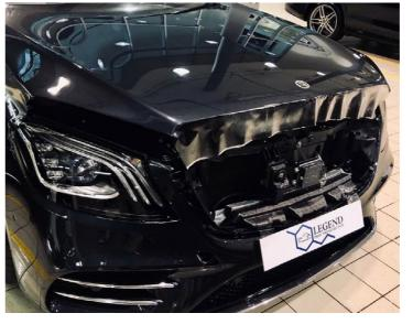
Align the film on the bumper. You can temporarily tack the corners to ensure that the film stays in place.
