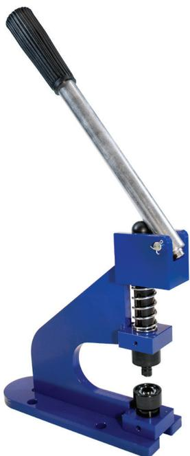
Stable multi-functional eye press to eye PVC banners and firm textiles. The construction units of the hand press are cut with a precision laser, that makes a modern and simple design possible. Due to the small clearance of the press stamp, plastic grommets can be processed in one step, punch and press. The Platinum Duo eye press is delivered with a 12 mm tool for plastic grommets. With other tools it is possible to use EMBLEM metal grommets from 3,4 mm to 11 mm.
